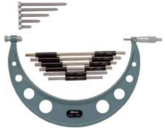
• Interchangeable Anvil Micrometer • A Mitutoyo non-digital micrometer that accepts easily interchangeable anvils to enable a wide variety of measurement, such as tubing thickness, shoulder-edge distance and rivet height. A ratchet stop guarantees repeatable measurement.
