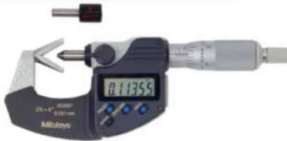
• Digimatic V-ANVIL Micrometer • It measures the outside diameter of cutting tools (such as taps, reamers, end mills) which have three or five flutes. V-anvils with a centreline groove are available for measuring the pitch diameter of taps by the single-wire method.
