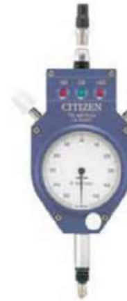
• Dial indicators with data output • Analogue indicators with limit LED's, output and even 0.5um resolution from CITIZEN Japan
